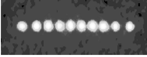
Figure 23.4. Linear crystal with ten ^{40}\text{Ca}^+ ions imaged by a CCD system. The fluorescence light near 397 nm is observed while the ions are excited by laser light at 397 nm and 866 nm. The trap used for this experiment is shown in Fig. 23.1b.
